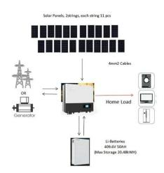
hybrid inverter is a cutting-edge device that ingeniously integrates the functionality of both a ...
