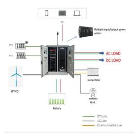
the base station while storing excess energy in the battery. At night, the energy storage system discharges to supply power to the base station, ...
