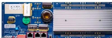
RS485 Communication between battery and inverters Band rate 9600bps RS485 Interface Communication between parallel pumps or BMS and PC Band rate 9600bps
