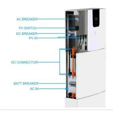
DC voltage into AC using high frequency PWM (6 kHz to 20 KHz) thus feeding the 50-Hz transformer which Boost it to 120V/220V AC.
