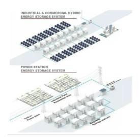
Battery energy storage connects to DC-DC converter. DC-DC converter and solar are connected on common DC bus on the PCS. Energy Management System or EMS is ...
