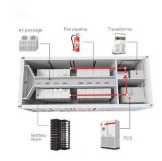
energy sources, the heart and the brain--Energy Storage Systems and ECO ControllerTM help rental companies and operators to deploy flexible power, ...
